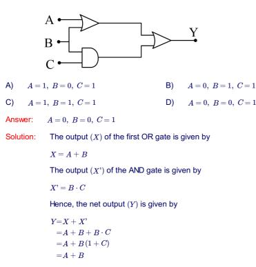
From the above calculation, it is clear that the value of the final output does not depend C. So, for the output to be zero, the values of A and B have to be zero.
