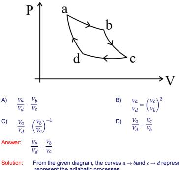
${\sf Q.1.} \qquad {\sf The} \ {\sf PV} \ {\sf curve} \ {\sf shown} \ {\sf in} \ {\sf the} \ {\sf diagram} \ {\sf consists} \ {\sf of} \ {\sf two} \ {\sf isothermal} \ {\sf and} \ {\sf two} \ {\sf adiabatic} \ {\sf curves}.$
