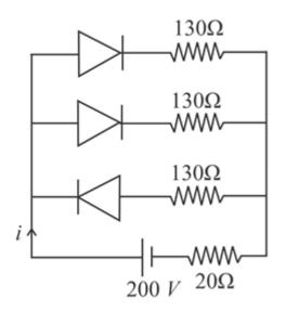
Effective resistance is given as  $R_{eq} = \frac{160}{2} + 20$  $R_{eq} = 80 + 20 \Rightarrow R_{eq} = 100 \Rightarrow i = \frac{200}{100} = 2A$
