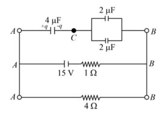
(A)  $24\mu C$ (B)  $120\mu C$ (C)  $10\mu C$ (D)  $6\mu C$ Ans. (A) Using  $i = \frac{15}{4+1} = 3 A$   $\therefore V_{AB} = i \times 4 = 12 V \therefore V_{AC} = V_{CB} = 6$  Volt  $\therefore q$  on  $4\mu F = CV_{AC} = 24\mu C$
