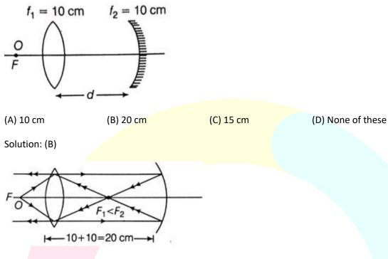
The final image will be at infinity only, if the foci of lens and mirror coincides. The situation could be understood on the basis of given diagram.
