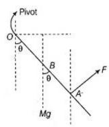
For equilibrium of the bar,  $F_{\text{ext}}^{\text{net}} = 0$  and  $\tau_{\text{ext}}^{\text{net}} = 0$ taking torque about pivot O,  $OB \times Mg + OA \times F = 0$   $\Rightarrow -OB Mg \sin \theta + OA. F \sin 90^{\circ} = 0$ (clockwise) (anti-clockwise)  $\therefore IF = \frac{1}{2}Mg \sin \theta$  $\Rightarrow F = \frac{Mg \sin \theta}{2}$
