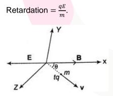
It is clear that the speed of the particle will be minimum when its component of velocity is along the direction of electric field.
