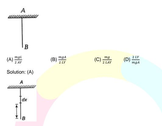
Consider a small section dx of the bar at a distance x from B. The weight of the bar for a length x is,  $W = \left(\frac{mg}{L}\right)x$ .
