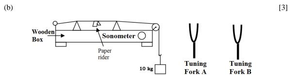
The diagram above shows a wire stretched over a sonometer. Stems of two vibrating tuning forks A and B are touched to the wooden box of the sonometer. It is observed that the paper rider (a small piece of paper folded at the centre) present on the wire flies off when the stem of vibrating tuning fork B is touched to the wooden box but the paper just vibrates when the stem of vibrating tuning fork A is touched to the wooden box.
