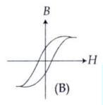
The graph of B is graph of soft ferromagnetic material which is we use to consist of electromagnets and transformers.
