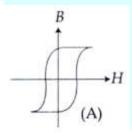
Graph A is hard ferromagnetic material substance.
