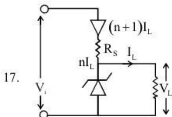
Voltage drop across zener diode is  $V_L$  so voltage drop across  $K_s$
