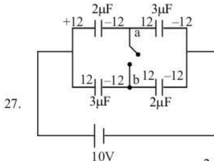
$$\text{for upper link } C_{\text{eq}} = \frac{6}{5} \mu\text{F}$$
